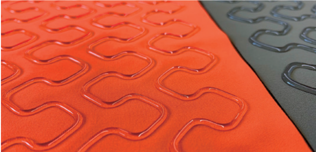
DPW DPW is our original dispensing application which directly print the polymer on the fabric. Applicable for various products.
